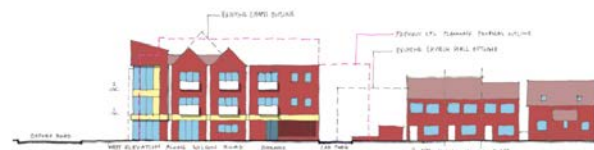
2018 Preliminary Sketch Option 1 (small gables) – mass reduced, greater separation from houses on Wilson Rd
